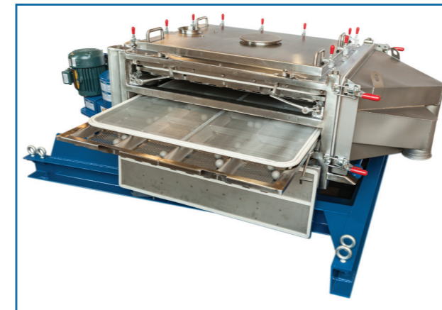
▲ Modified Apex™ with hinged discharge chute and easy to remove top panel
