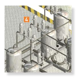
Compressed gases which come into direct contact with ingredients, the finished product, packaging materials, storage vessels or the manufacturing machinery, are termed critical and require sterile filtration to safeguard against a potential contamination of the brew.
