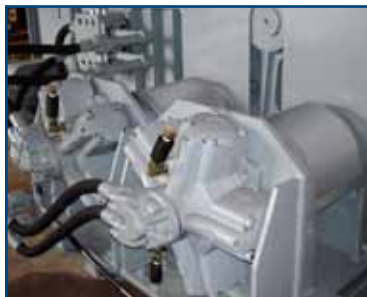
CH clutch mounts between motor and winch
