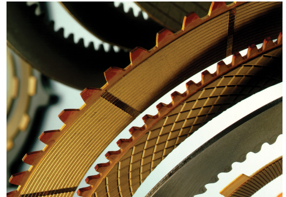
Friction-faced and high-carbon steel separator discs
