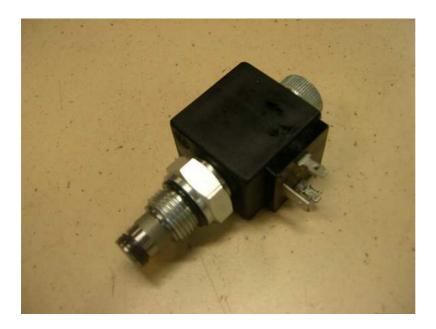
2way-2pos solenoid valve incl. magnet
