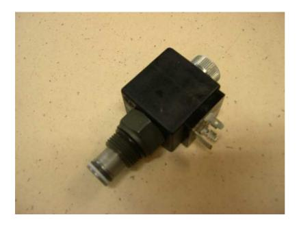
2way-2pos solenoid valve incl. magnet - 12V Hirschman (DIN) conta
