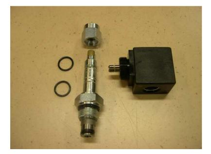
Set consists of 1pc valve SV-08-2-1NC M 1pc nut 2pc O-ring 1pc magnet 12V S2-12-13,25-M24 24V S2-24-13,25-M24
