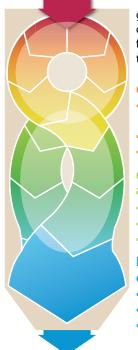
The Gyratory Reciprocating Motion gradually diminishes along the length of the machine to an elliptical path and finally to a nearly straight line motion at the discharge end.
