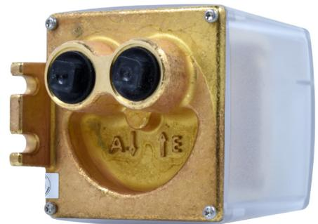
When performing filter membrane tests, the difficult part of the task is disposing of the test fuel. The Meter Monitor solves that problem completely. The flush and the test fuel are both returned to the fuel system and are never exposed to air, rain, or other contaminant sources. No buckets, funnels, or fuel spills. The Meter Monitor has two 1/8" NPT connections.
