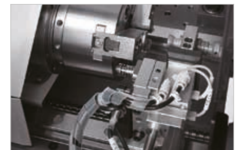
Transfer between spindles (SP1 and SP2)
