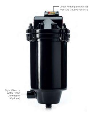
The Facet VF-21SB/22SB, when configured as a filter water separator, is an economical, compact housing designed to remove water and solids from aviation fuels. Both interior and exterior surfaces of the carbon steel body are epoxy coated to protect against corrosion. This sturdy, single cartridge housing is easy to maintain and requires only 2" (51 mm) base clearance for cartridge change out.
