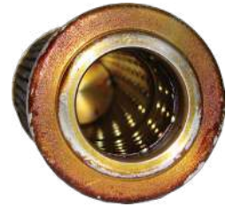
Varnish deposits on filter element (GE Frame 6B)
