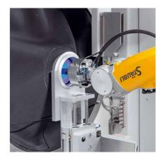
Up to four blasting guns are included with the base system. Additional blasting guns that can be added as an option.
